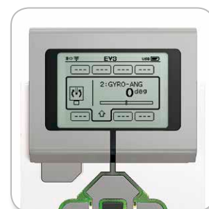
Port View with Gyro Sensor
